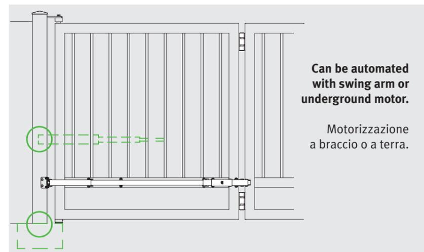
Can be automated with swing arm or underground motor.
