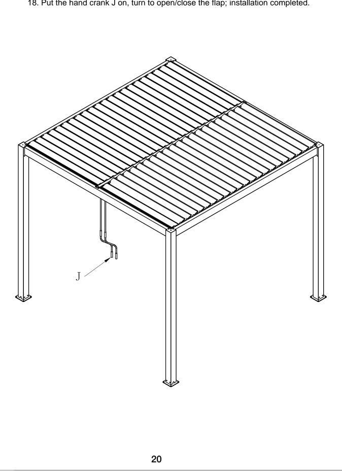
18. Put the hand crank J on, turn to open/close the flap; installation completed.
