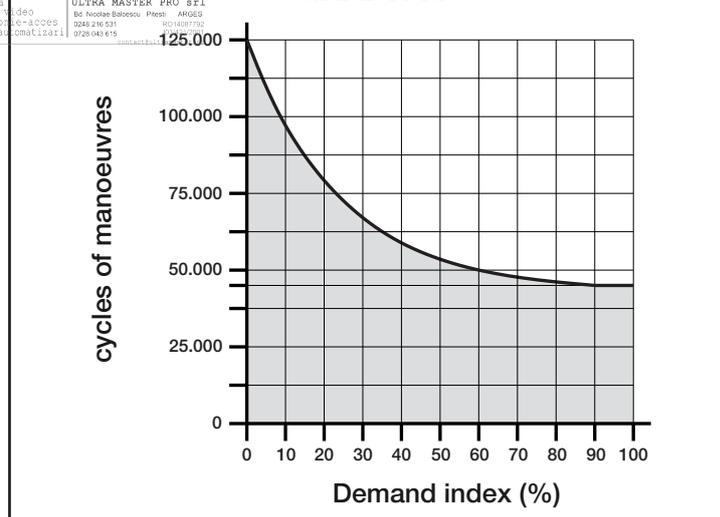
**Example of calculation of durability of a Wingo WG5024 gear motor (refer to Table 2 and Graph A):**
